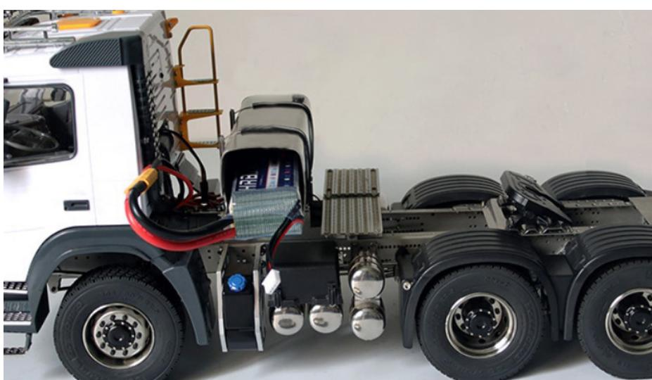
3. Insert the battery into the compartment then connect it to the XT60 plug(Not;Ensure that the radio is turned on before the battery is connected,for safety reasons
