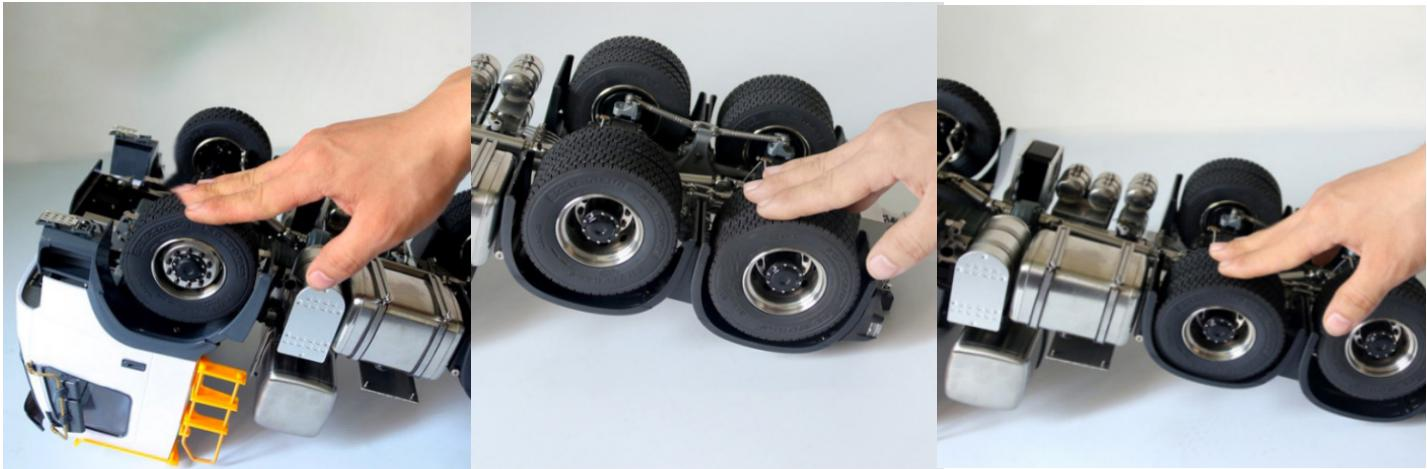
1. Grab the tire with a little force by hand AT this time there is only one tire on the side has force
